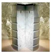
Cementation through the use of specially formulated grouts provides the means to immobilise radioactive material that is on solids and in various forms of sludges and precipitates/gels (flocks) or activated materials.
