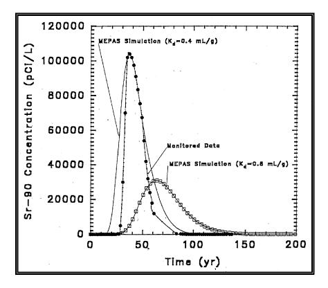
Figure 4.3. Example illustrating MEPAS  ${}^{90}$ Sr calibrations with K<sub>d</sub> equaling 0.4 and 0.8 ml/g and several monitored-data points.
