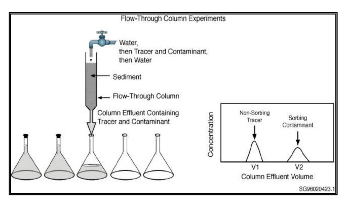
**Figure 3.3**. Procedure for measuring a column K<sub>d</sub> value.
