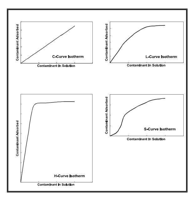
Figure 2.2. Four types of adsorption isotherm curves shown schematically in parlance of Giles *et al.* (1974).
