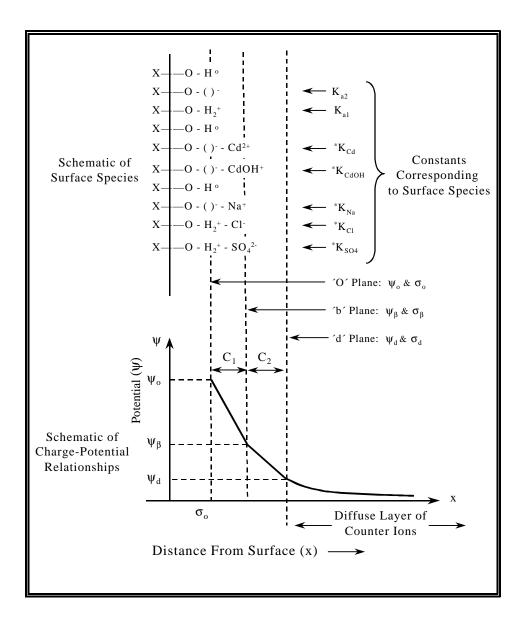
**Figure 5.4**. Schematic representation of the triple layer model showing surface species and surface charge-potential relationships. [Taken from Peterson *et al.* (1987a). Brackets in the *o* plane indicated deprotonated surface sites.]
