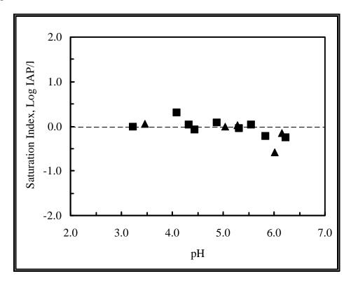
**Figure 5.2**. Saturation Indices calculated for rutherfordine (UO<sub>2</sub>CO<sub>3</sub>) as a function of pH for solution analyses from Sergeyeva *et al.* (1972). [Adapted from WATEQ4 modeling results of Krupka *et al.* (1983). The filled square and triangle symbols refer, respectively, to solutions analyses from 25 and 50<sup>°</sup>C experiments by Sergeyeva *et al.* (1972)]
