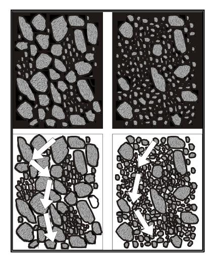
**Figure 2.3.**Schematic diagram for conceptual model of water distribution in saturated (top two figures) and unsaturated soils (bottom two figures) suggesting differences in the unsaturated flow regime (indicated by arrows) for soils with varying texture. [The two figures on left represent coarse-textured soils, whereas the two figures on the right represent fine-textured soils. Soil particles, air, and water are shown, respectively, in stippled gray, white, and black.]
