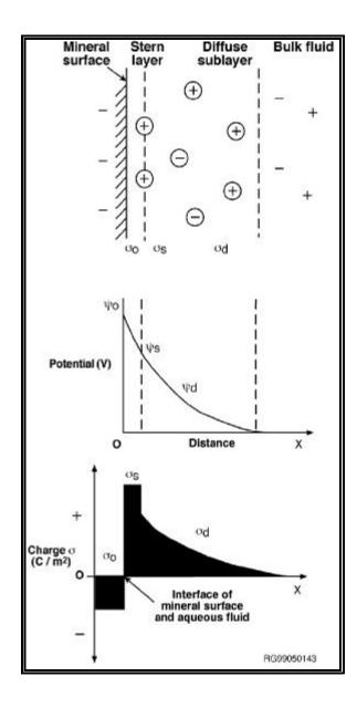
**Figure 2.1.** Diffuse double layer and surface charge of a mineral surface.  $(\sigma_o, \sigma_s, and \sigma_d$  represent the surface charge at the surface, Stern layer, and diffuse layer, respectively;  $\psi_o$ ,  $\psi_s$ , and  $\psi_d$  represent the potential at the surface, Stern layer, and diffuse layer, respectively.)
