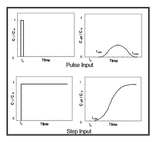
**Figure 3.4.** Schematic diagram showing the relative concentrations of a constituent at the input source (figures on left) and in the effluent (figures on right) as a function of time for a pulse versus step input.  $[C_o, C_i, and C_{eff}$  refer, respectively, to the concentration of the constituent at  $t_o$  and the concentrations of the constituents in the input and effluent.]
