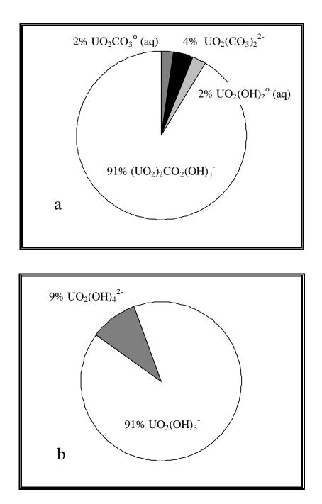
**Figure 5.1.** Distribution of dominant U(VI) aqueous species for leachates buffered at pH 7.0 by local ground water (Figure 5.1a) and at pH 12.5 by cement pore fluids (Figure 5.1b). [Adapted from MINTEQA2 modeling results of Krupka and Serne (1998).]
