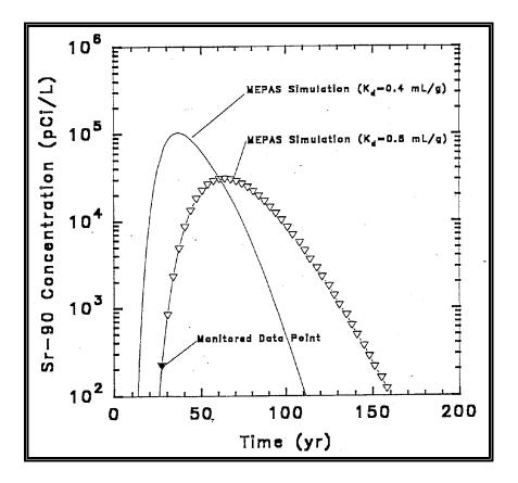
**Figure 4.2.** Example illustrating a MEPAS  $^{90}$ Sr calibration with  $K_d$  equaling 0.8 ml/g and 1 monitored-data point.
