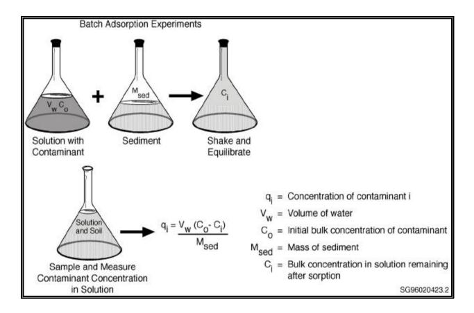
Figure 3.1. Procedure for measuring a batch K<sub>d</sub> value (EPA, 1991).
